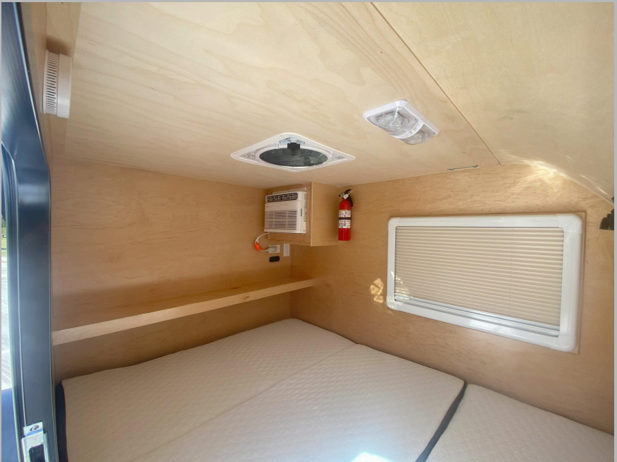
Interior with Standard Window, Air Conditioner, Roof Vent
